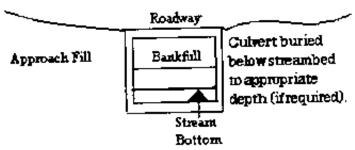
In all other counties: Culverts greater than 48 inches in diameter will be buried at least one foot below the bed of the stream. Culverts 48 inches in diameter or less shall be buried or placed on the stream bed as practicable and appropriate to maintain aquatic passage, and every effort shall be made to maintain the existing channel slope. The bottom of the culvert must be placed at a depth below the natural stream bottom to provide for passage during drought or low flow conditions.
